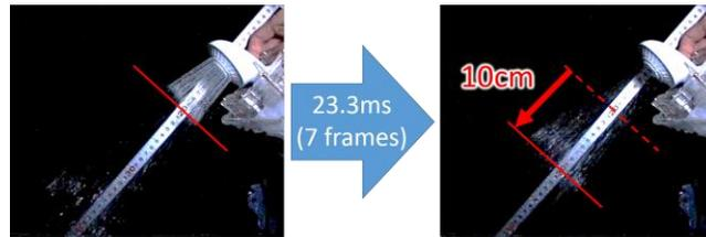
Figure 7 Speed measurement of water flow
