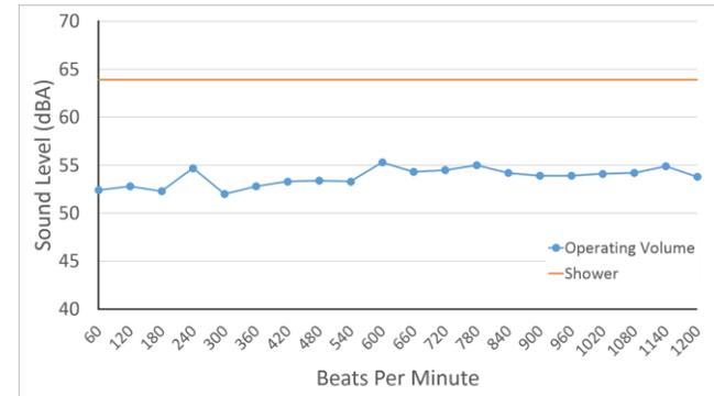
Figure 9 Sound level of operating volume for 60-1200 BPM. "Shower" is the background noise of the water from the shower.
