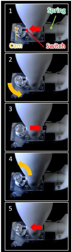
Figure 4 Cam mechanism
