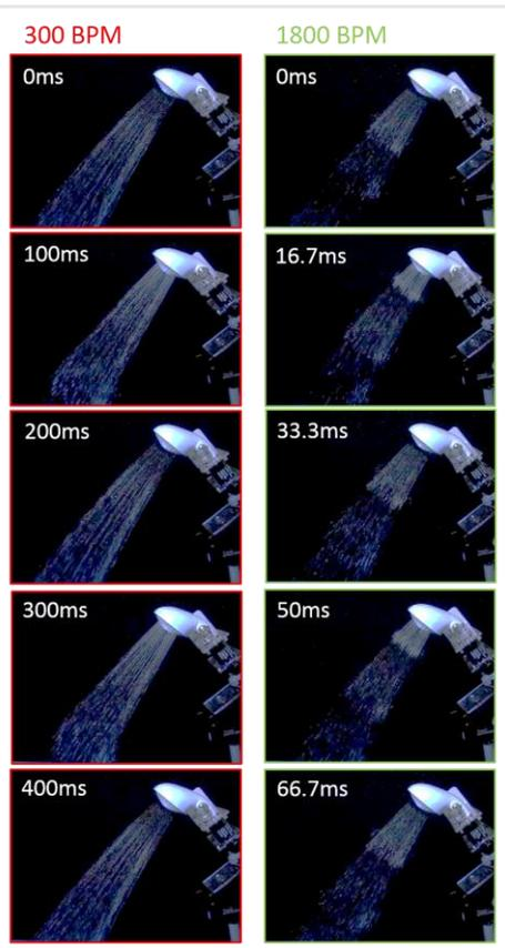
Figure 6 Water flow observed by high speed camera (300 BPM, 1800 BPM)
