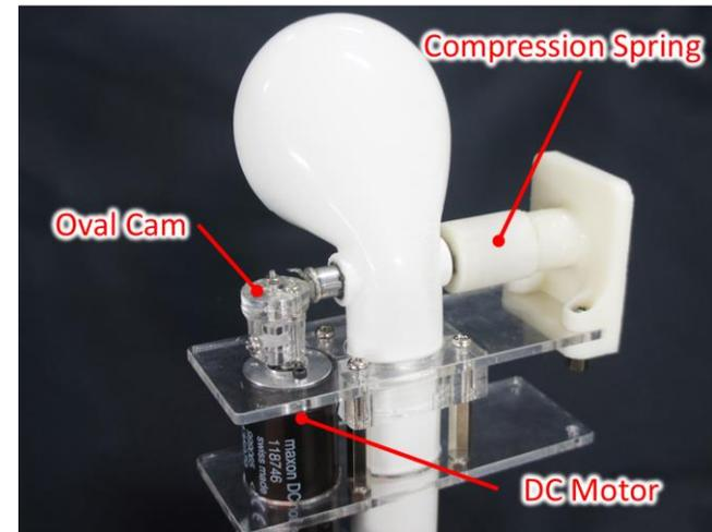
Figure 2 Prototype device: a mechanical switch on the showerhead is pushed by a camshaft.
