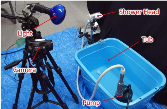
Figure 5 Setup to measure the bandwidth and latency
