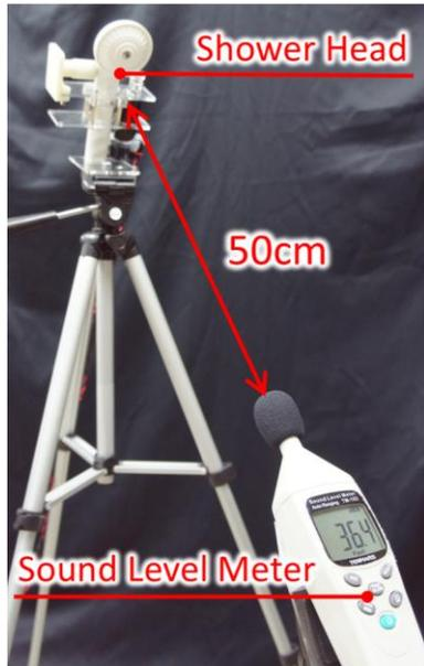
Figure 8 Setup to measure the sound level of operating volume: The sound level meter was located 50 cm away from the showerhead.
