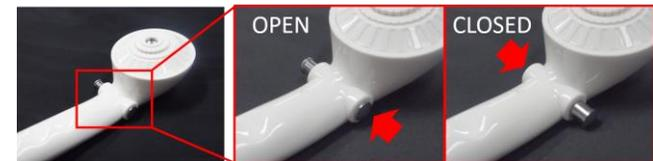
Figure 3 Mechanical switch on the showerhead: pushing the switch by 8 mm can switch the water flow (open / closed)
