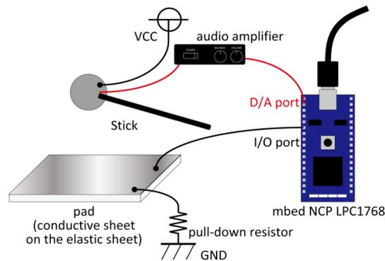
**Fig. 3.** System configuration
