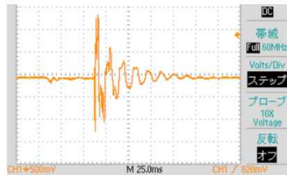
Fig. 4. The waveform of the hitting measured by the accelerometer.
