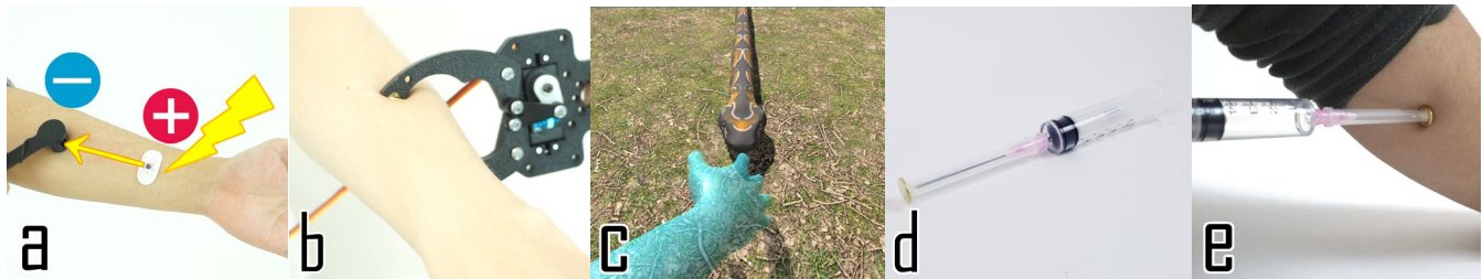
Figure 1 Electrical stimulation increases the intensity of physical stimulation. (a) Electrical stimulation while hitting the skin. (b) Gripper-type physical object with servomotor and an electrode attached at the tip. (c) VR scene of being bitten by a snake. (d) An electrode attached at the tip of a syringe. (e) Training to get used to injection.
