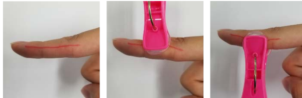
Fig. 2. Skin deformation occurs in the extension direction when the clothespin is attached at the back side of the hand, and in the bending direction when the clothespin is attached from the palm side of the hand.
