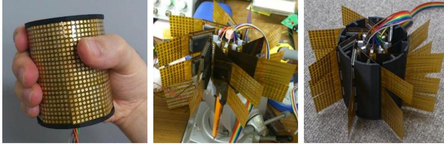
**Fig. 4.** Cylindrical electrocutaneous display, internal connection and construction.
