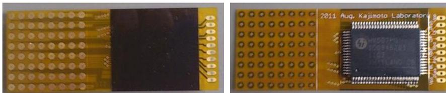
**Fig. 3.** Flexible electrode unit with 64 electrodes and one driver IC.
