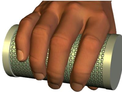
**Fig. 1.** Image of cylindrical electrocutaneous display.
