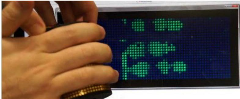
**Fig. 5.** Touch sensing by impedance measurement during stimulation.
