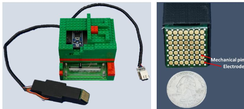
**Fig. 1.** Appearance of prototype device (Left: overall image; right: array of pins and electrodes)
