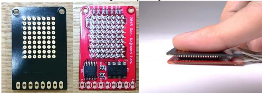
**Fig. 5.** High-density TVSS. (Left) electrodes, (center) sensors, (right) combined, side view.
