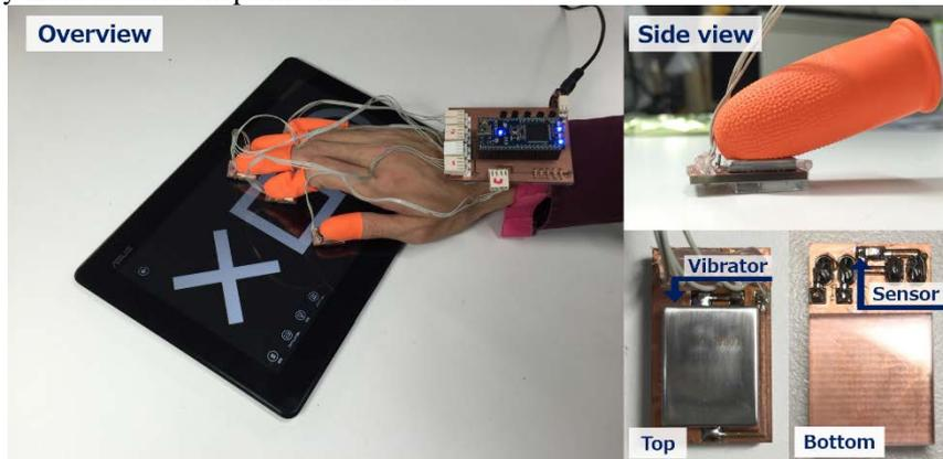
**Fig. 1.** Overview of the prototype using a vibrator and a sensor unit for each finger.
