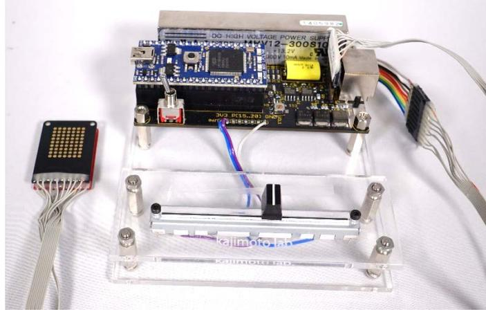
**Fig. 4.** Electro-tactile stimulation device for a single finger.
