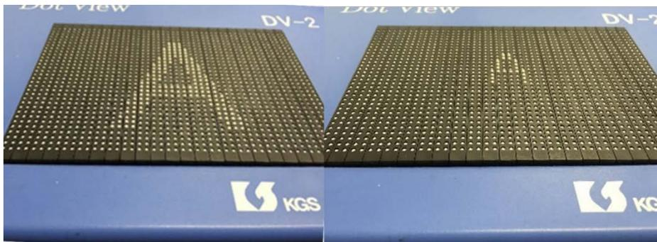
**Fig. 2.** Displayed character on the tactile display; (left) large condition, (right) small condition.
