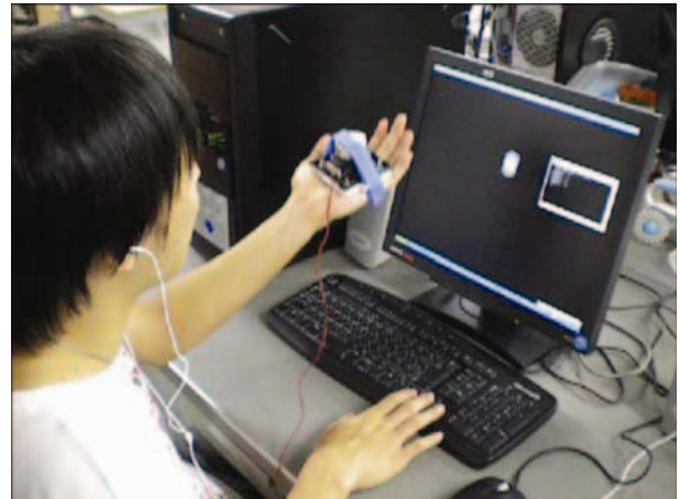
Figure 5. Experiment 2: Measurement of the vibratory threshold during forearm motion
