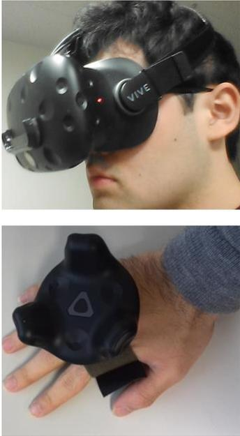
Figure 2: HMD (top) and Vive tracker (bottom) used to reflect the hand position in the VR space.
