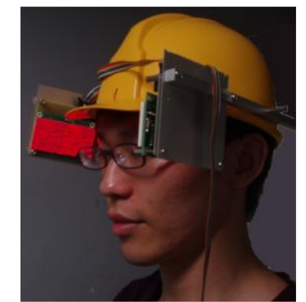
Fig.6 A User Put on the Peripheral Display (The Bottom Display is omitted)
