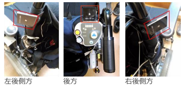
Fig. 3 Installation image of the sensor electrode
