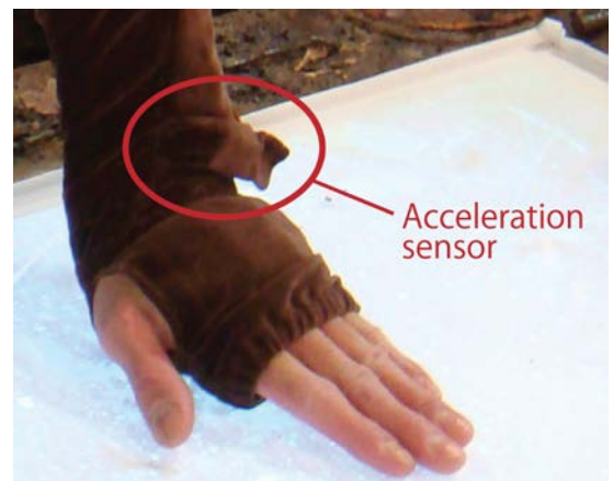
Fig. 5 The position of acceleration sensor
