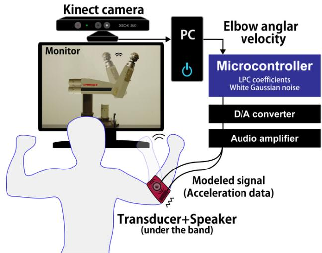
Figure 6. Hardware setup of the prototype system. In AR Jointonation system, we will use an HMD instead of the monitor to superimpose virtual robot arms on the user's arms.
