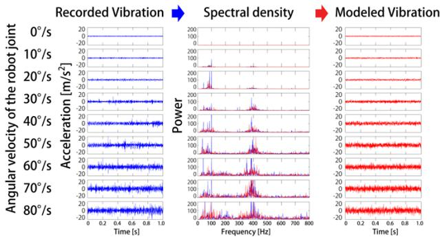
Figure 5. Recorded vibration (left), example of LPC-modeled vibration (right), and overlaid spectral density (center).
