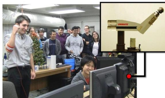
Figure 2. Overview of the prototype system. The user (left) feels as if his arm became a robot arm on the monitor. The robot arm model tracks the user's right forearm.
