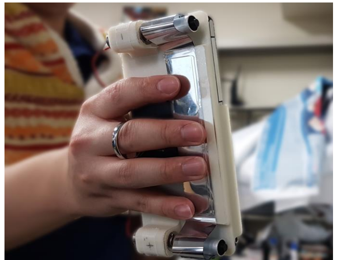
Fig. 1 Prototype of the proposed device: this device presents vibration using belt-winding mechanism
