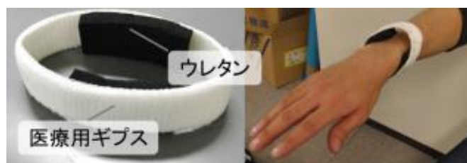
Fig.2 Hanger Reflex device for wrist
