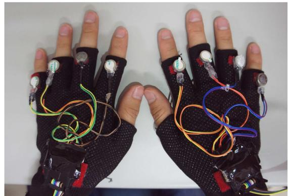
Figure 1. Glove-type tactile device
