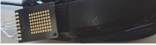
Figure 2. Electro-tactile display used in the experiment.
