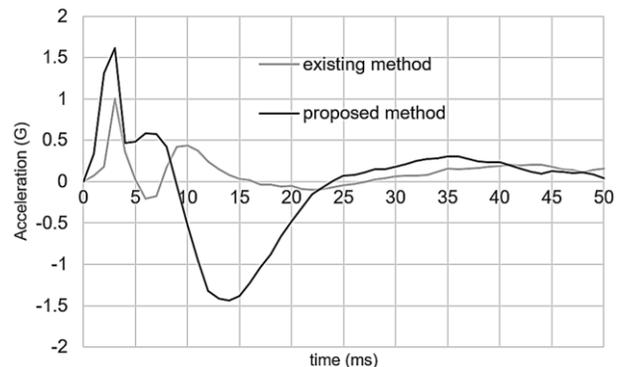
Figure 4 Time response of each vibrotactile actuator
