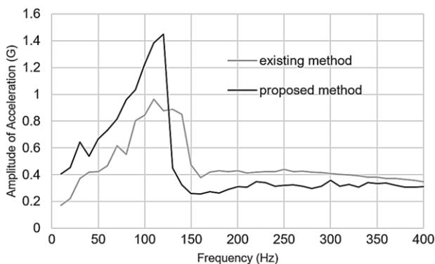
Figure 5 Frequency response of each vibrotactile actuator
