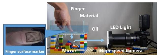
Figure 1. Measurement system[6]
