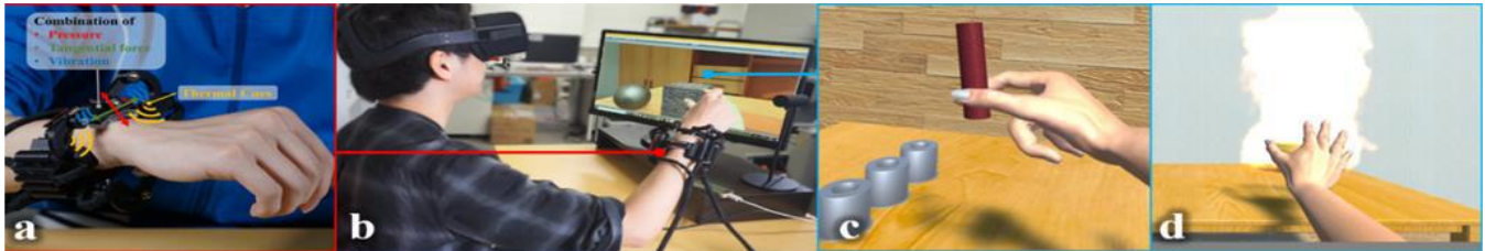
Figure 1: Images showing (a, b) the haptics display, (c) the touching and grasping of an object, and (d) thermal cues
