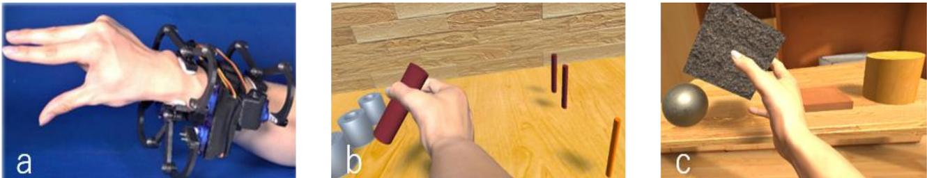
Figure 1: (a) Haptics Display (b, c) Touching and Grasping an objects
