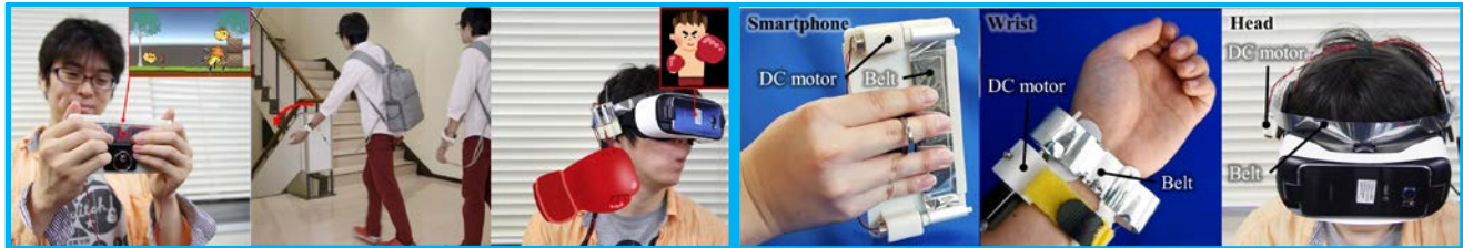
Figure 1: Our belt-driven method enables vibration and force feedback in the game for smartphone, walking navigation by presenting a rotational force to the wrist, and being hit sensation in VR fighting game by presenting and force sense (left). Smartphone, wrist, and head-type device(right).
