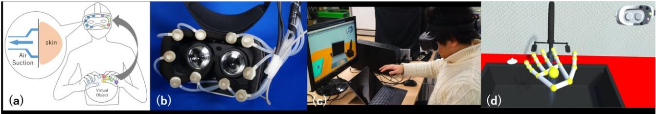
Figure 1: (a) Concept images of Haptopus, (b) Haptopus, (c) playing application, (d) user's view
