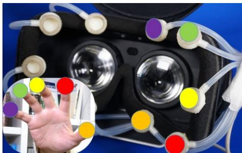
Figure 3: Haptic Mapping of Transferring Touch Sense of Hand to Face
