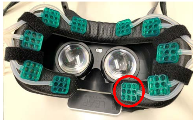
Fig. 3 Suction unit attached to the HMD. In this experiment, only the part surrounded by a red circle was used.
