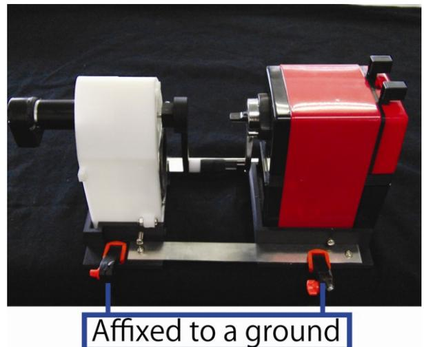
Fig. 3 Experimental figure: Each device is connected by paper tape. Both are affixed to the surface
