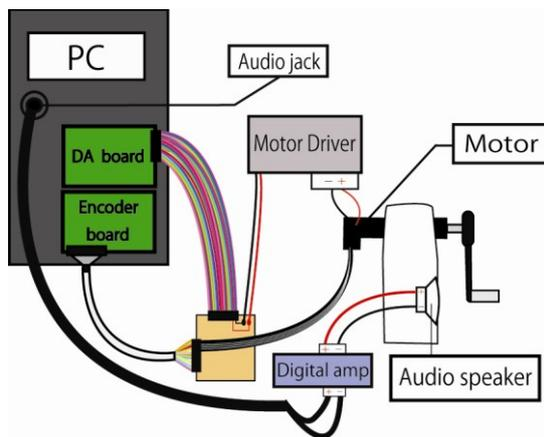
Fig. 2 System configuration
