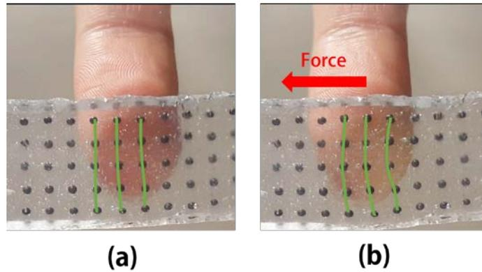
**Figure 5.** Deformation of marker-containing gel in the lateral direction (a) without force (b) with force
