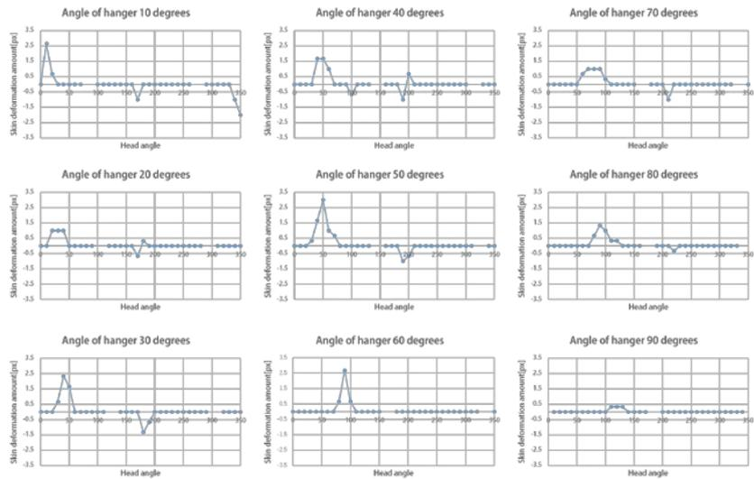
**Figure 9.** Gel deformation elicited by a wire hanger placed on the left front temporal region of a head model
