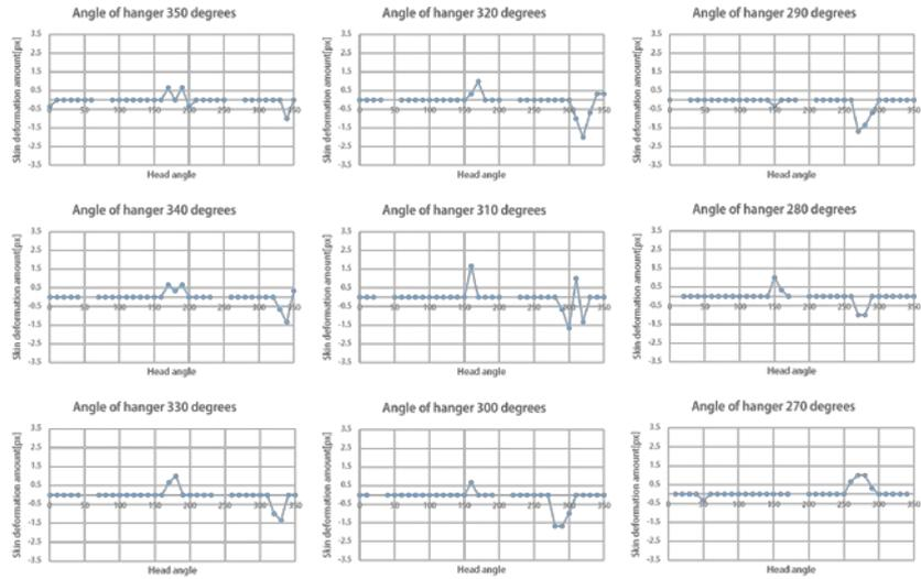
**Figure 8.** Gel deformation elicited by a wire hanger placed on the right front temporal region of a head model
