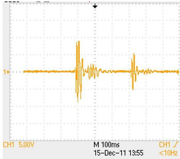
**Figure 2.** Actual output voltage from the audio speaker
