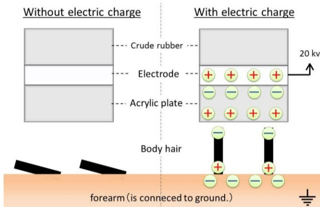
Figure 1: Principle of the prototype device
