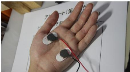
Figure 6: Attached positions of electrode seals
