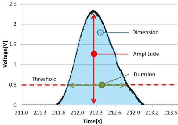
Figure 4: A typical waveform of SCR during the trial
