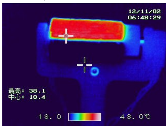
Figure 4: Working device observed by thermal camera
