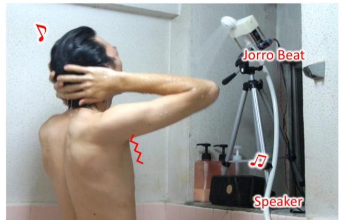
Fig. 1 “Jorro Beat”: water flow from the showerhead synchronizes music and beats out a rhythm on a wide area of the user’s body.
