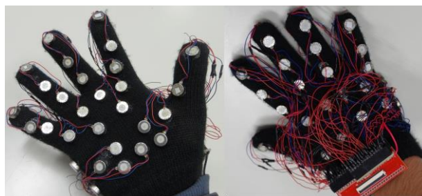
Fig. 1 The haptic glove with 52 linear resonant actuators
