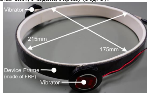
Fig. 1 The developed device for the head: the device is made of FRP, so it deforms elastically when the user wears it.
