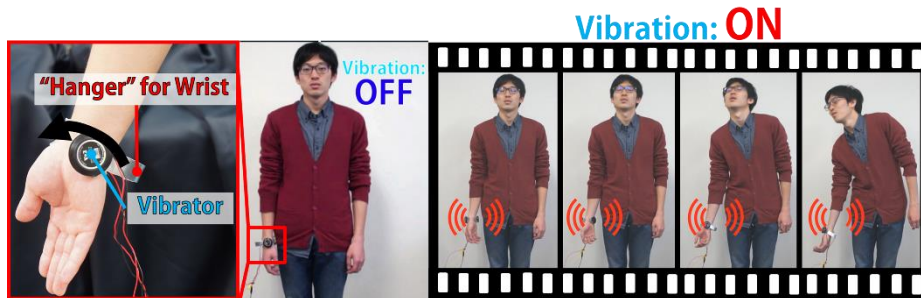
Fig. 1 Presenting the vibration on the wrist under the hanger reflex: The force caused by the hanger reflex is enhanced, and it induces the wrist rotation
