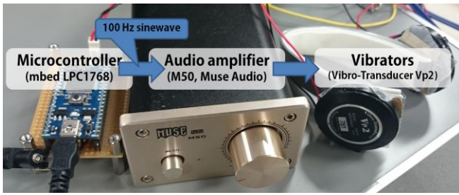
Figure 2. Configuration of the Hanger Reflex device attached with vibrators
