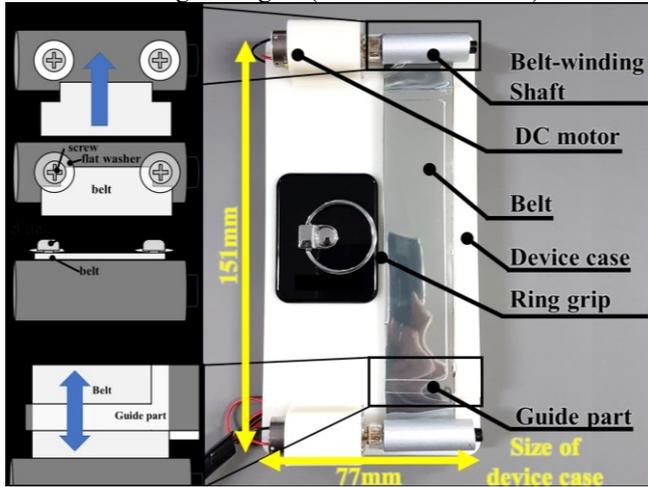
Figure 2. Configuration of the prototype
