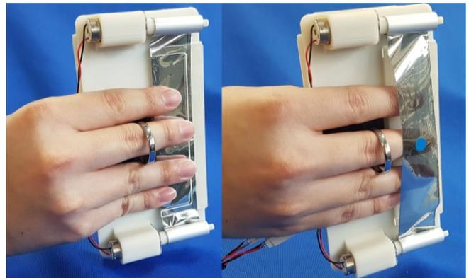
Figure 1. Overview of the prototype. (Left) Vibration is transmitted to the fingertip by touching on the belt in “On belt condition”, and (Right) to instep of the fingers by covering fingers in “Under belt condition”
