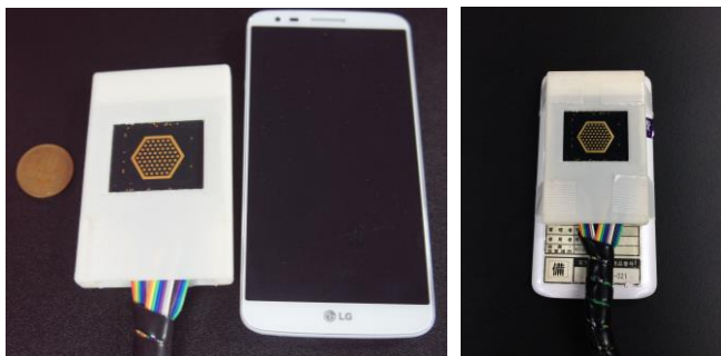
Figure 2. Prototype. The tactile display is attached on the back side of the smartphone.
