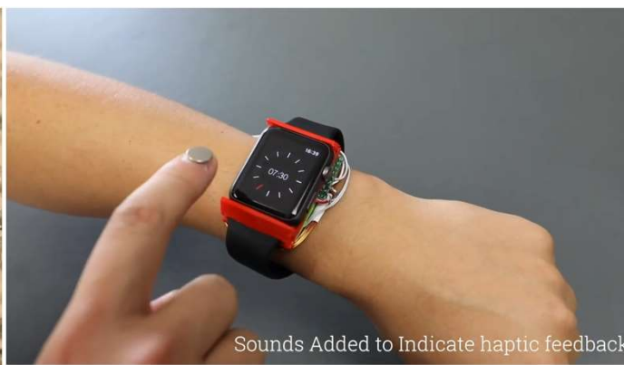
(CHI2019) Magnetips: Combining Fingertip Tracking and Haptic Feedback for Around-Device Interaction Jess McIntosh, Paul Strohmeier, Jarrod Knibbe, Sebastian Boring, Kasper Hornbæk https://www.youtube.com/watch?v=-lBZ2xzx2jU スマートウォッチの下に電磁石、指に磁石。磁石は位置検出にも用いる
