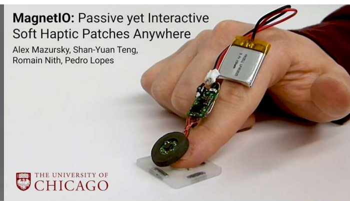
(CHI2021) MagnetIO: Passive yet Interactive Soft Haptic Patches Anywhere Alex Mazursky, Shan-Yuan Teng, Romain Nith, Pedro Lopes https://www.youtube.com/watch?v=hsCo3g3Jk-y0 環境側に磁石埋め込み、指にコイル
