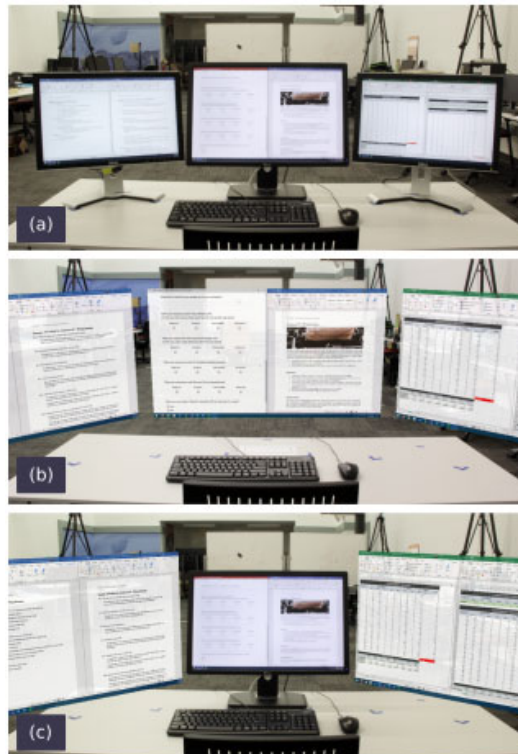
Figure 2: (a) Physical condition had three monitors side-by-side; (b) Virtual condition had three monitors rendered through HoloLens; (c) Hybrid condition combined a central physical monitor with two peripheral virtual monitors.
