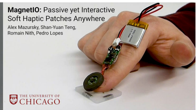
(CHI2021) MagnetIO: Passive yet Interactive Soft Haptic Patches Anywhere Alex Mazursky, Shan-Yuan Teng, Romain Nith, Pedro Lopes https://www.youtube.com/watch?v=hsCo3g3JKy0 環境側に磁石埋め込み、指にコイル
