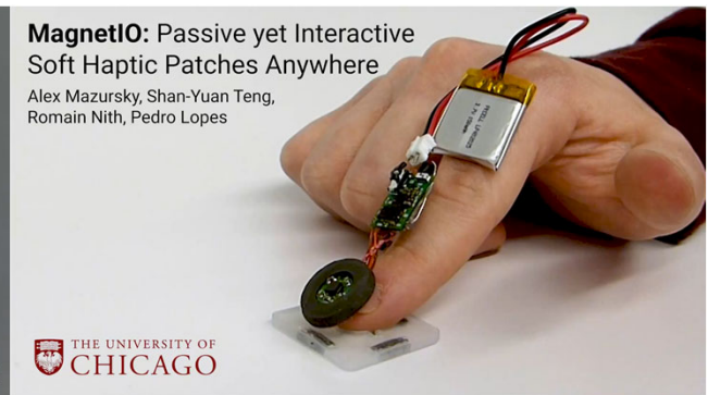
(CHI2021) MagnetIO: Passive yet Interactive Soft Haptic Patches Anywhere Alex Mazursky, Shan-Yuan Teng, Romain Nith, Pedro Lopes https://www.youtube.com/watch?v=hsCo3g?IKy0 環境側に磁石埋め込み、指にコイル
