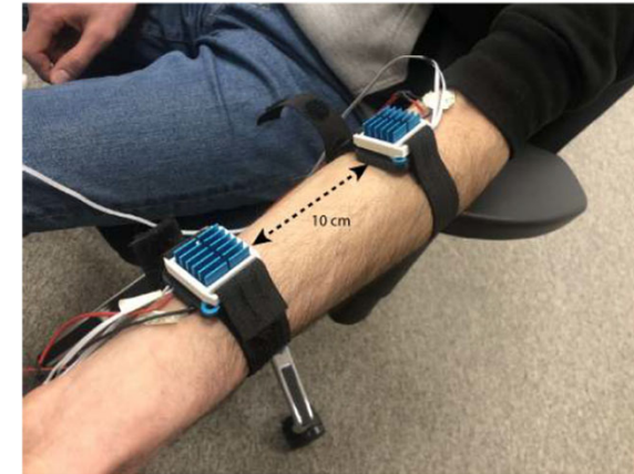
Fig. 5: Study setup of Peltiers attached with a wristband to the forearm
